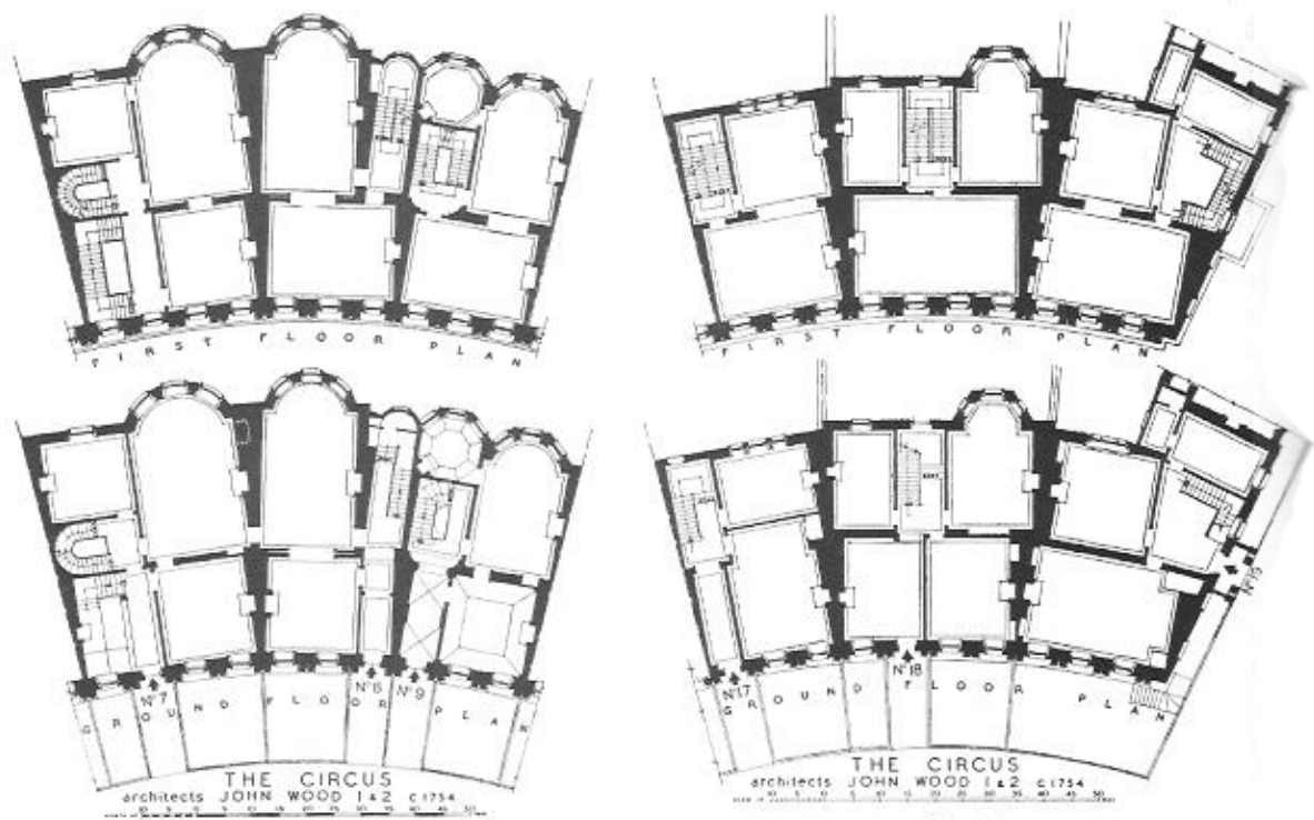
Figure 8. Although the façade is of uniform appearance, the plan forms at The Circus in Bath are each individual, reflecting the requirements of the original owners for whom they were built (W. Ison, The Georgian Buildings of Bath from 1700 to 1830 (Kingsmead, 1980) p. 98. Image courtesy of Bath Preservation Trust). Within most of the houses, a plan type can however be identified. The party walls are wedge shaped in order that the rooms could remain square.
